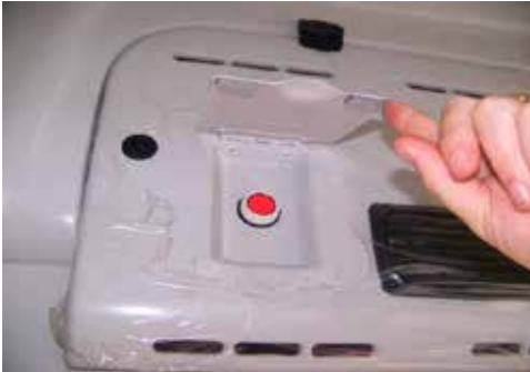
Figure 2-4 Emergency door open button front door - internal
