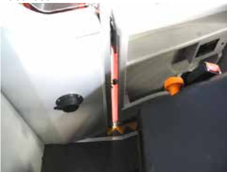
Figure 2-2 Emergency alarm on left hand side of driver
