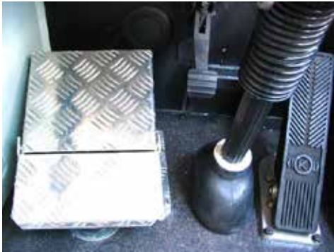
Figure 2-1 Emergency alarm under flip-up foot rest
