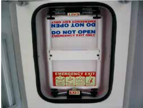
Figure 2-11 Roof Hatch Emergency Exit
