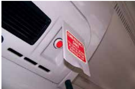
Figure 2-5 Emergency door open button rear door - internal
